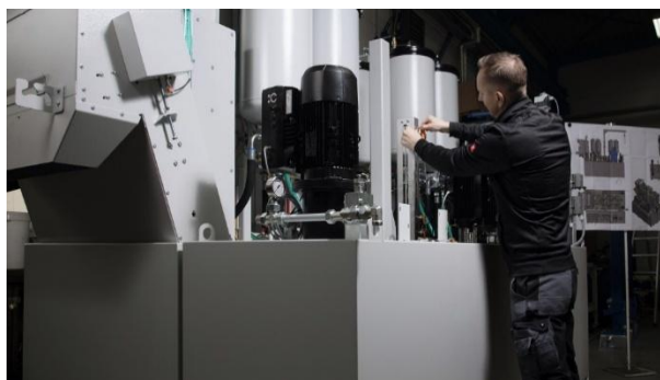
Employees of Lehmann-UMT GmbH during the installation of the filter domes
